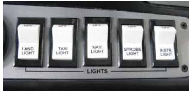
Figure 11. – Lights switches panel
